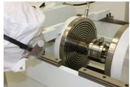
Emissions testing using clean, dry nitrogen or helium is used to shell test and seat leak test the valve in both directions, when appropriate.
