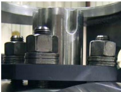
Live-loading maintains proper pressures on application-specific stem packing and anti-extrusion rings.
