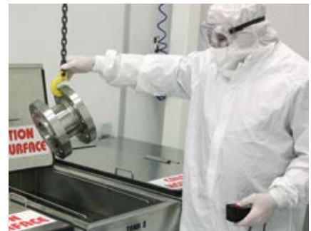
Precision cleaning—such as oxygen, aqueous and ultrasonic cleaning—of valves and critical parts reduce non-volatile residue to acceptable ISO standards.
