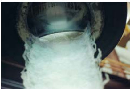
After years of use in a tough polymer application, this valve was returned to MOGAS Service facility for maintenance. Minimal repair was required before being re-installed.
