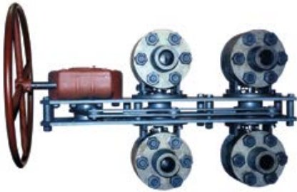
This special linkage allowed one flow line to run while the other was isolated. This enabled the operators to open two valves and close two valves in a single operation.
