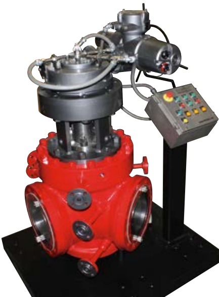
This 8-inch ASME 600 Class 4-way switching valve maintains >90 percent flow area of full bore during mid-stroke. It also has the flexibility of valve placement (horizontal or vertical mounting position) to help minimize capital piping expenditures.
